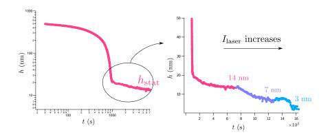
Non-zero stationary thickness h<sub>stat</sub> depends on the Marangoni forcing.
