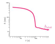
Non-zero stationary thickness  $h_{\text{stat}}$
