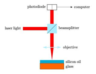
Low power laser (30 mW max). Completely wetting liquid on a smooth surface.
